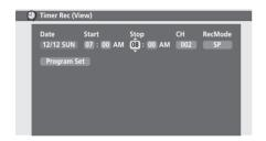
3 Set a new Stop time for the timer recording. Use the  $\leftarrow/\Rightarrow$  buttons to select the hour or minute field. then use the  $\uparrow/\downarrow$  buttons to change the time.
